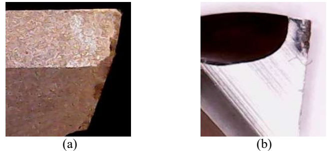
Figure 6. Microscope digital image Endmill wear (a) Relief face (b) Rake angle face
